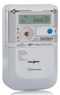
Sx401 G3-PLC are three-phase and single-phase smart meters designed for measurement of electrical energy of residential consumers, with integrated G3-PLC modem and switching module for remote reading and power management. Wide range of measurement values including power quality data in combination with large capacity of load profiles makes this meter a key tool for utilities for making insight in overall condition of low voltage network. Robust G3-PLC technology in
